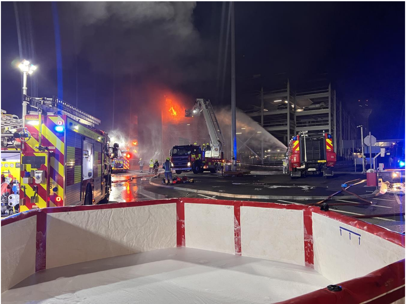
Figure 9 Water damn in use
